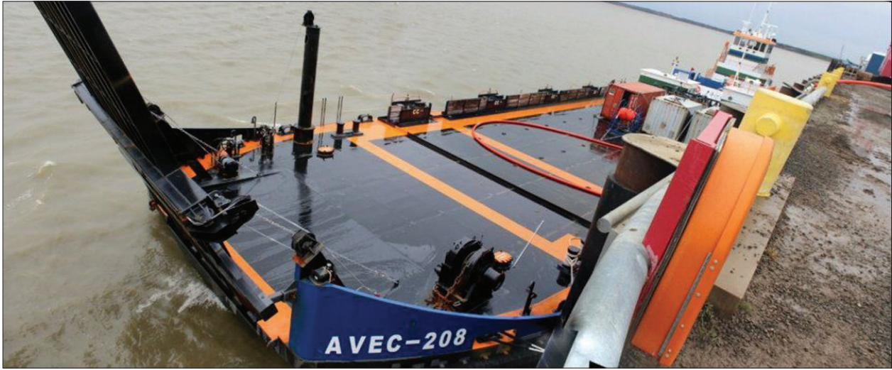
These vessels made their first fuel delivery of 1.1 million gallons to Nushagak Electric Cooperative in Dillingham, transferring four barge loads from a line-haul barge. The vessels can pump 34,000 gallons of fuel per hour. More information and photos are available on the Vitus Marine Facebook page.
