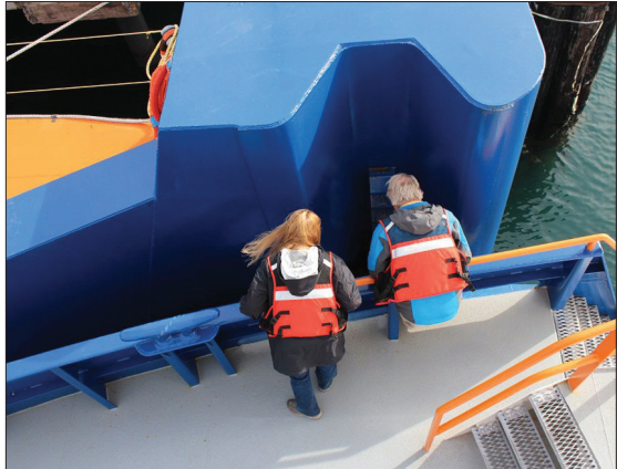
The vessels use an articulated-tug-barge system that increases maneuverability and efficiency. Amy Murphy and Graham MacDonald watch the tug's notch and pin connect to the barge.
