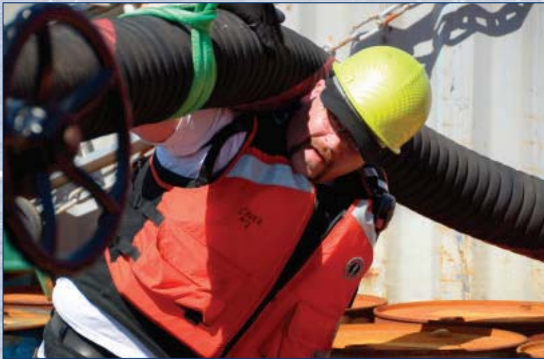
Isaac Sargent guides a 6-inch hose to the header on the Cavek , where fuel from the tanker Orestina will flow.
